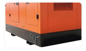
Reinforced connectors between the upper part of the canopy and the base frame. Optional removal of the selected parts of the canopy facilitates maintenance.
